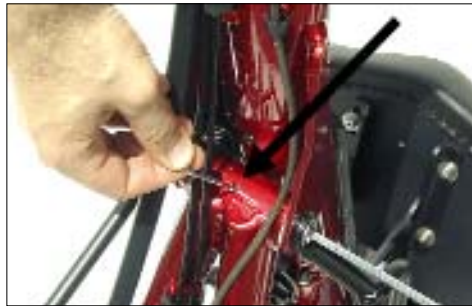
You can prevent the axle from turning by inserting a thin metal rod in the hole of the axle.
