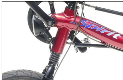
The suspension of the front wheel is integrated in the steerer tube.
