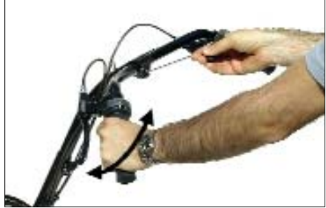
After you have undone the clamping screw you can adjust the handlebars.
