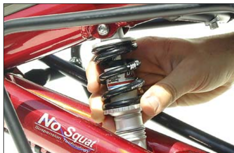
Turning the adjustment ring for the pre-load.
