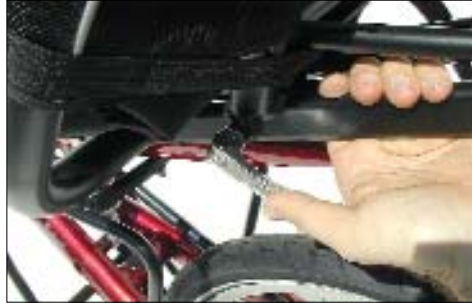
The quick release levers must be closed firmly. Hold the seat frame with your fingers to enhance your thumb's power.
