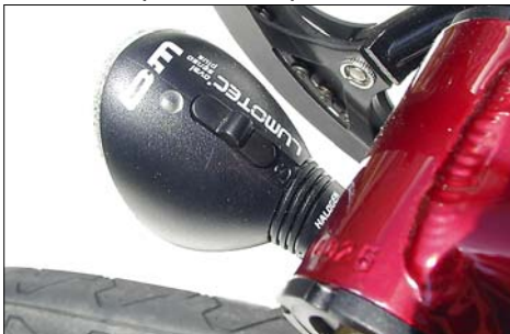
You switch on the hub generator light system with the integrated switch at the front light.
