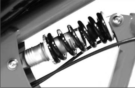
*Suspension element DV-22 with fixed damping rate.*
