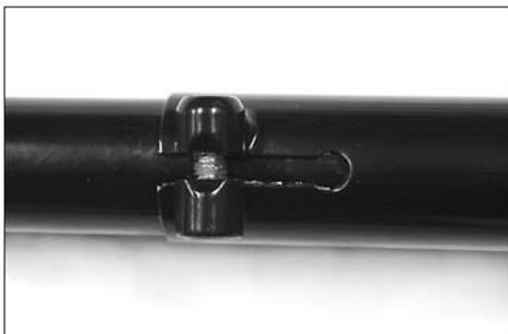
The end of the upper stem half must not be visible in the clamping slot.
